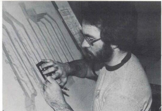
Designer Dennis McGarrahan draws a switch that will allow two central processors to share the same 'Winchester' disc drive
