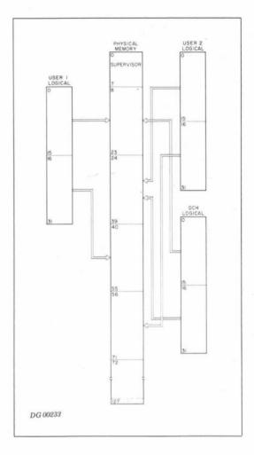
In order to manage memory efficiently, the operating system makes use of the validity and write protect features of the address translation hardware, if possible. The next figure shows a two-user configuration where these features are used.
