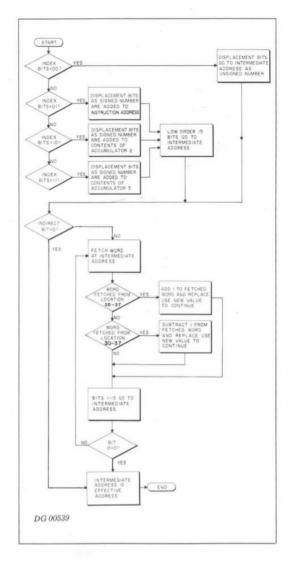
An effective address is always 15 bits in length. This means that an instruction which uses the effective address calculation can address any one of  $32,768_{10}$  words. This gives rise to the concept of an address space, which, in the NOVA 4, contains 64K bytes or 32,768 2-byte words.
