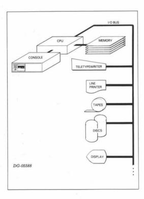
Due to the general-purpose design of the NOVA 4, the type, size, and number of memory modules and I/O devices have no effect upon the internal logical structure of the CPU. This chapter deals with the addressing of information and the logical representation of information within the CPU, and is unaffected by those portions of the system outside the CPU.
