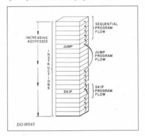
Because the program counter is 15 bits in length, it can address 32,768 separate memory locations. The next memory location after 777778 is location 0, and the location before 0 is location 777778. If the program counter rolls from 7777778 to 0 in the course of sequential operation, no indication is given and processing continues with the location addressed by the updated value of the program counter.
