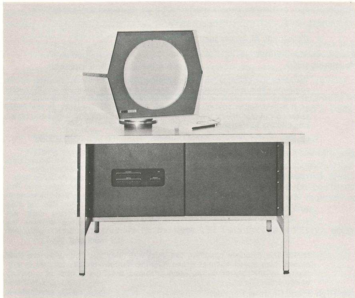
Precision CRT Display with Light Pen
