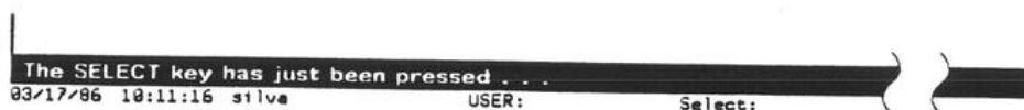
Figure 3.4 The status line changes from Tyi to Select: after you've pressed the SELECT key. If you don't want to select anything, press SELECT again.
