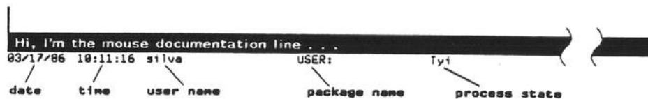
Figure 2.2 The line with the date and time in it is called the status line . It's your best immediate information on what the machine is doing.
