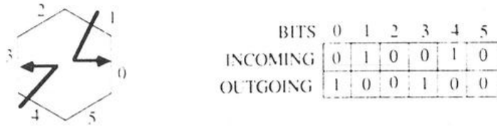
Figure 3.3: Hexagonal cells with six incoming bits for particle direction and six outgoing bits for particle direction
